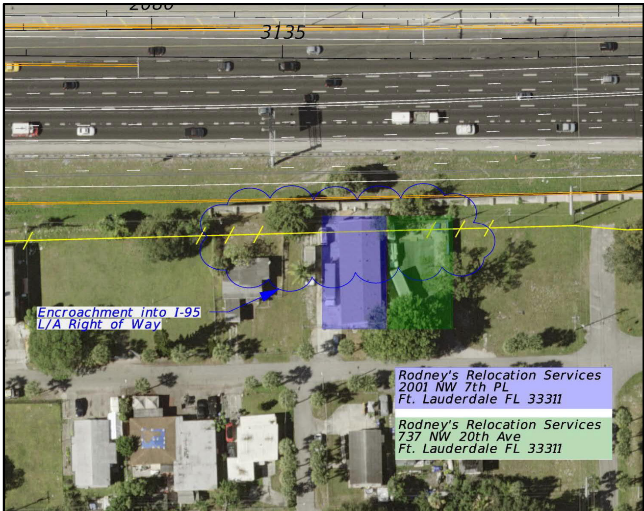
Figure 29 | Right-of-Way Encroachments along East Side of SR9/I-95
